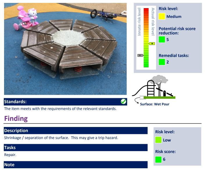
Wet pour edges are shrinking and lifting, creating potential trip points - repair.
