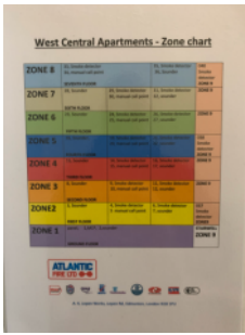
Fire alarm zone information
