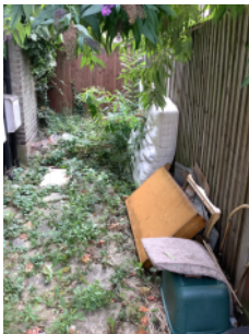
Mattress and other combustibles near to the building
