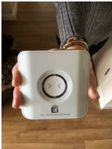
Remote wireless fire alarm controller installed in each flat
