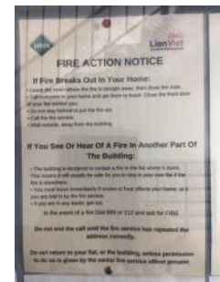
Inappropriate Fire Action notice by entrance door- reflecting Stay Put
